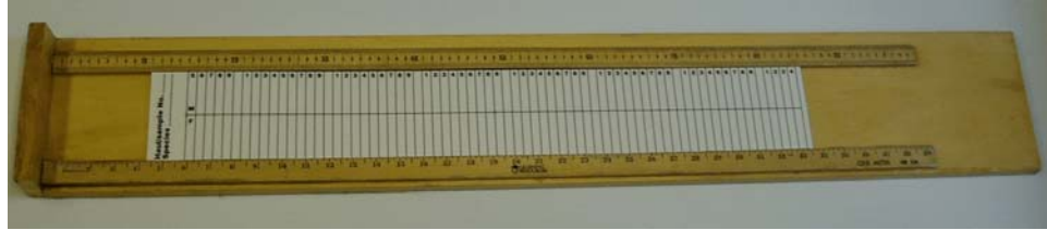
Figure 18. Measuring board and length frequency tally sheet used to record fish length frequency data during the SMAST Trawl Survey. Fishermen measure individuals of a given species directly over the insert on the measuring board. The tally sheet is labeled with species, trip, haul and other information. Totals for each length are then transcribed onto the length frequency data log (Figure 20).
